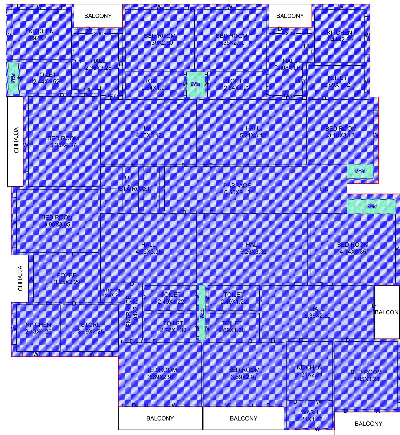
FIRST FLOOR PLAN (Existing) (SCALE 1:100)
