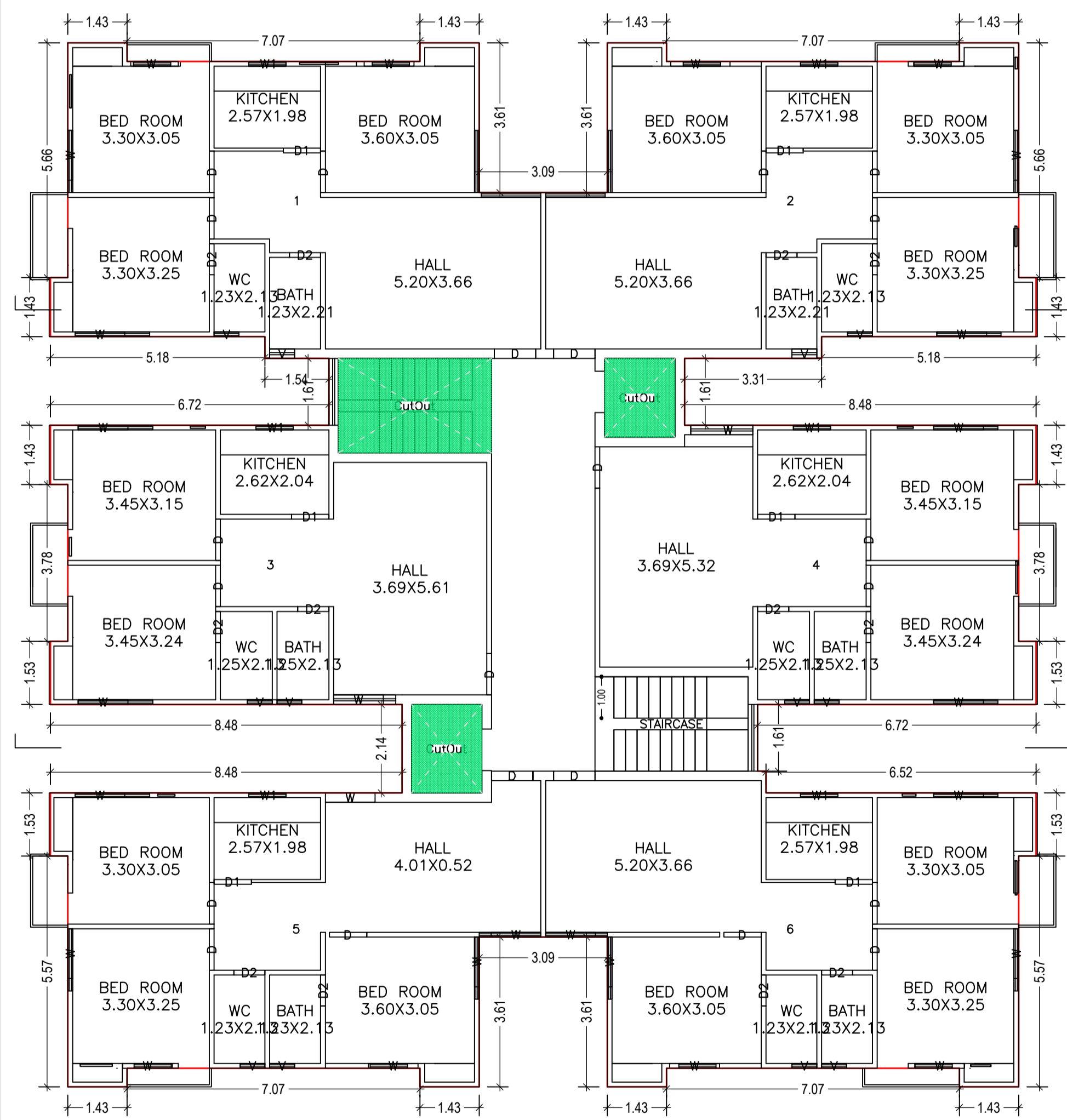
GROUND FLOOR PLAN (Proposed) (SCALE 1:100)
